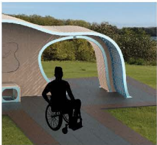
A continuous rubberized surface provides a stable, slip-resistant foundation that supports wheelchair users
