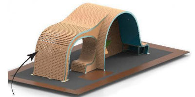
Intermittent cladding pattern on this side to let in some light
